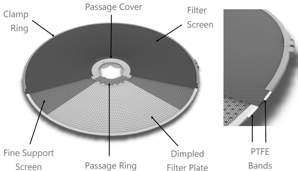
Each filter plate assembly consists of a filter plate, a support screen, and a filter screen. The passage cover holds the fine support screen and the passage ring in place while the filter screen is mounted with an outer clamp ring, sealed with a PTFE band. The slightly dished form of the filter plate assures complete drainage of the filtered liquid.
